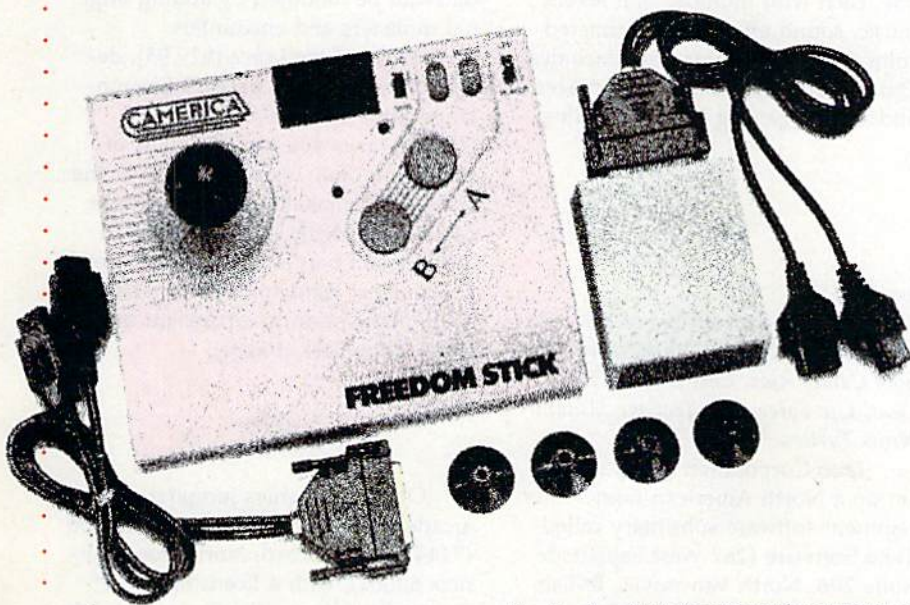
The Freedom Stick from Camerica operates as a wireless remote control.
